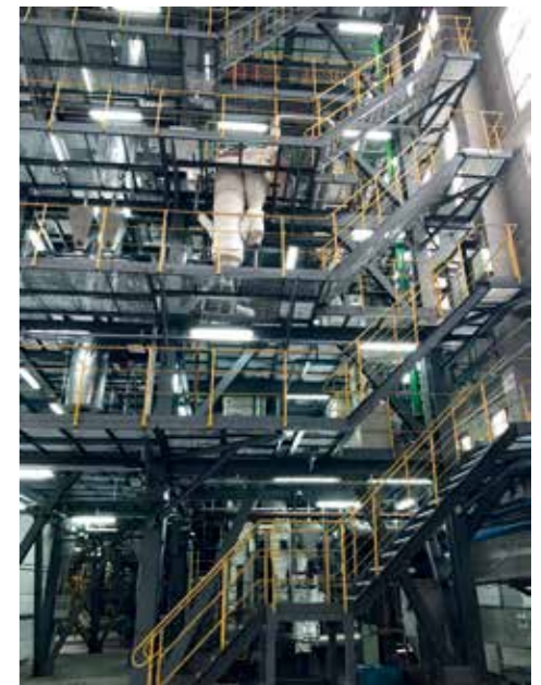
MW 级煤粉预热燃烧试验平台 MW Test Platform of Preheating Pulverized Coal Combustion
