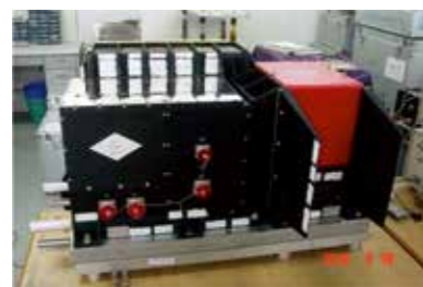
风云三号卫星红外分光计 InfraRed Atmospheric Sounder (IRAS) on-board FY-3 satellite
