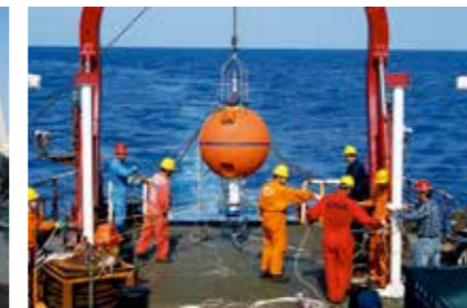
2010年西太平洋6100米深海潜标布放中 Deployment of the 6100 m deep ocean mooring in the western Pacific in 2010
